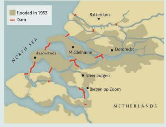
**Safety first.** The Delta Works, a response to the 1953 flood in the Netherlands, consists of a series of dams including a storm surge barrier across the Eastern Scheldt (*above, right*).
