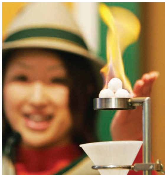
Great balls of fire! When methane meets water under high pressure and low temperature, it forms icy chunks that burn when lit.
