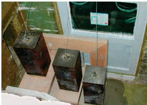
**Hot and heavy.** This Fraunhofer Institute test furnace measures how much weight treated wood can bear after burning.
